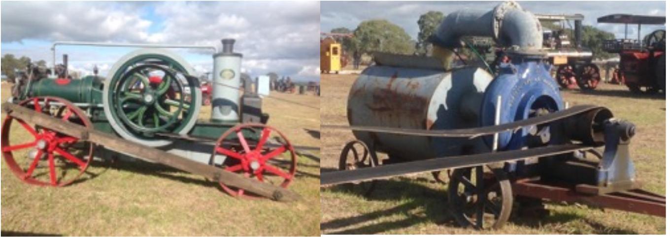
And as Heyfield members know this 1914 20 hp Ronaldson Tippet was restored by Jake and Mike Coleman in 2001 to drive the 9 inch, Robinson & Co unit that was used locally for diverting water at various sites. The pump was built in 1900, in its working life, worked 24/7.
