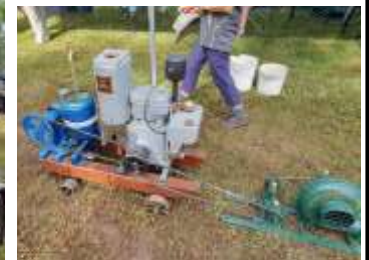
Jan's Ronaldson Tippett 1929, 2hp, type H engine rebadged in Australia by International Harvesting Company as "The Ideal Motor". It is displayed with a Nevertire Piston Pump.
