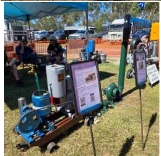
Jan's Ronaldson Tippett 1929, 2hp, type H engine rebadged in Australia by International Harvesting Company as "The Ideal Motor". It is displayed with a Nevertire Piston Pump.
