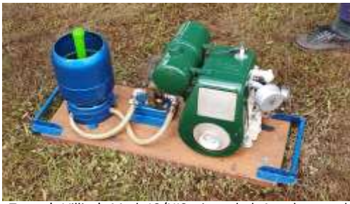
Trevor's Villier's Mark 12/HIS, air cooled, 4stroke petrol engine. Built between 1957 & 1966 in Ballarat.
