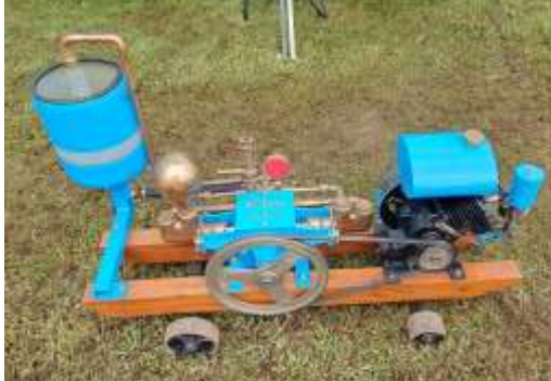
4 Cycle 1 3/4hp PT type engine teamed with a Marino pump. Displayed by Jan.
