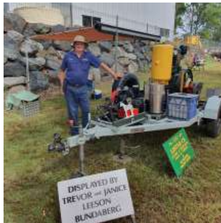
Jan's Ronaldson Tippett 1929, 2hp, type H engine rebadged in Australia by International Harvesting Company as "The Ideal Motor". It is displayed with a Nevertire Piston Pump.
