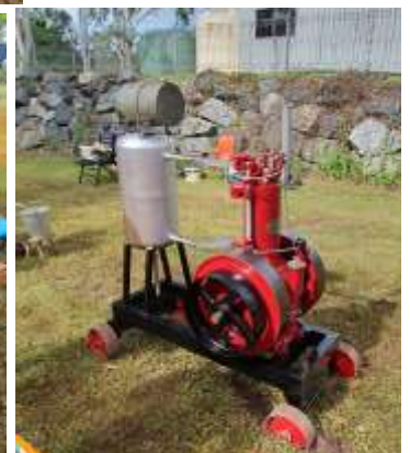
Indy's RanD 3 1/2hp diesel engine with a vertical water cooled tank and hvid injector system. It was manufactured by Rapson & Dutton in Brisbane in 1934. A limited number were made and this is engine 179. They were mainly sold around SE Qld and Northern NSW. It was used to run a generator on a poultry farm on the Sunshine Coast. This was the first time Indy has displayed this engine.
