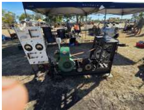
Trevor's 1949 Ronaldson Tippet Type "NA" vertical air cooled petrol engine with a Delco Remy generator.
