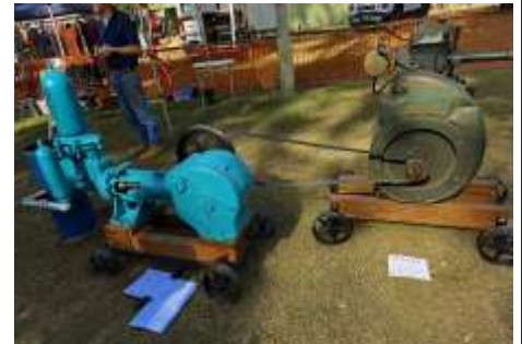
A Forrers Pump manufactured in Ipswich, Qld with a 1959 Lister Type "VA" engine
