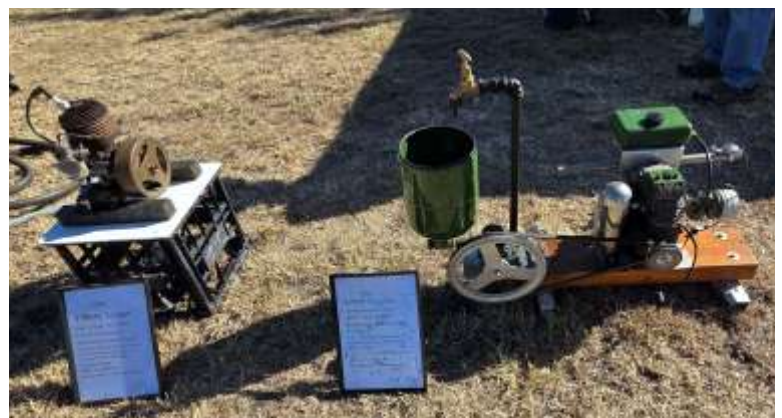
Neville's 1936 Villiers "Midget", single cylinder, 2 stroke petrol engine
