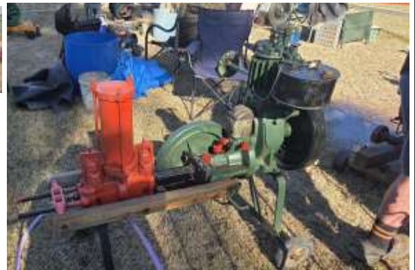
A Forrers Pump manufactured in Ipswich, Qld with a 1959 Lister Type "VA" engine
