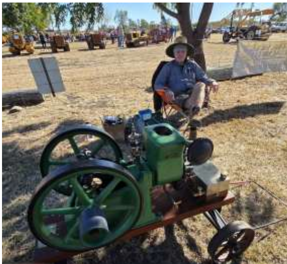
1919 "Chore Boy", 1 3/4hp gasoline engine. Owned and restored by Keith.
