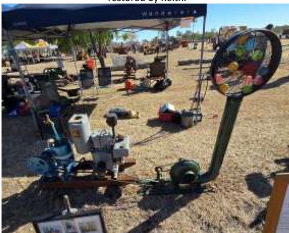
Above -2hp Type H engine manufactured by Ronaldson Tippet ( The Ideal Engine) with a Champion No1 Blower manufactured in the 1920's. Displayed by Jan.
