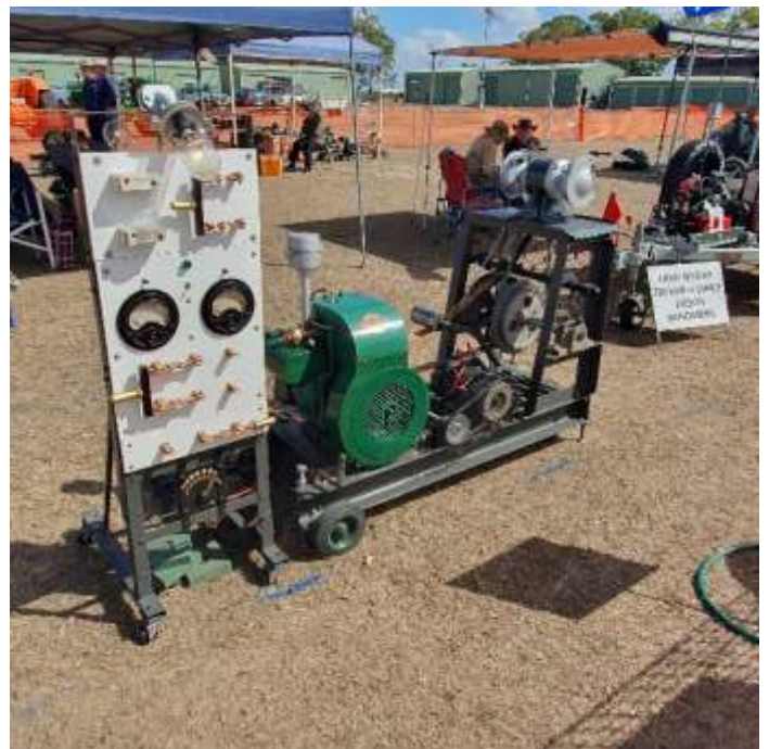
Trevor's Ronaldson Tippet Type NA engine built in Ballarat in 1949, operating a Delco Remy generator.
