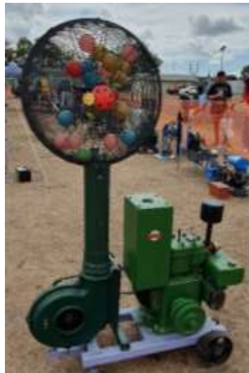
Jan's 2hp, 1943 Austral petrol engine working a P370 Southern Cross pump.
