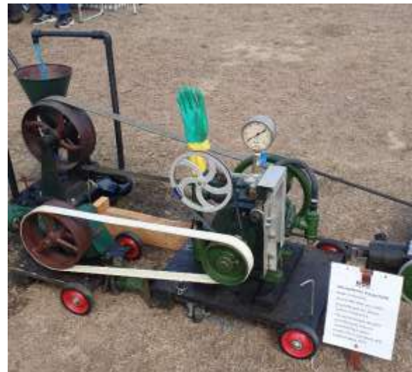
Ridd Milking Machine Vacuum Pump originally used in a Monto District Cream Dairy. This pump became obsolete when the dairy industry converted from cream production to bulk whole milk supply in about 1974.
