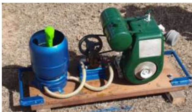
Trevor's Villiers Mark -12/1HS engine operating an FLH Bronze Gear Pump.
