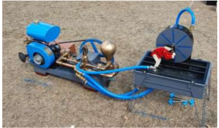
Ed's Marino engine operating a water feature.
