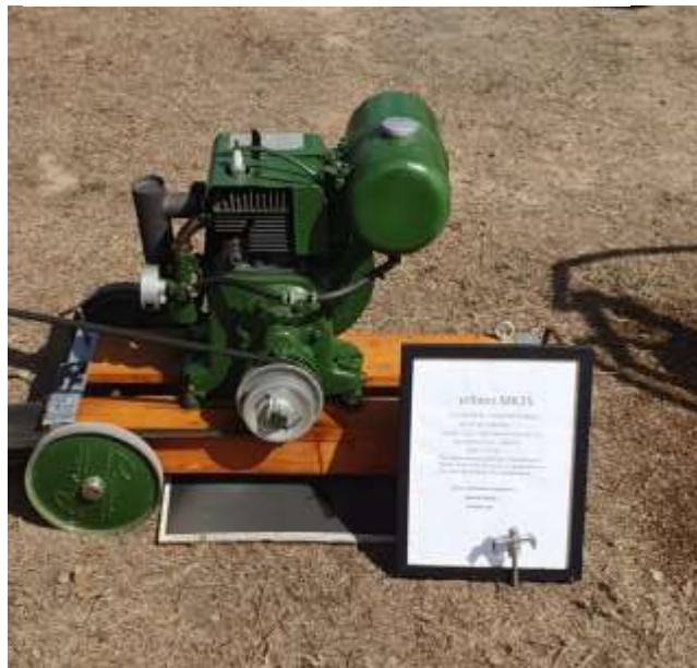
1940/41, 2.5 hp. Villiers MK25, 4 stroke, air cooled, petrol engine. This engine was purchased new in Bundaberg in 1941 by Herb Fritz who used it to pump water on his Lovers Walk family farm in Bundaberg, Qld.
