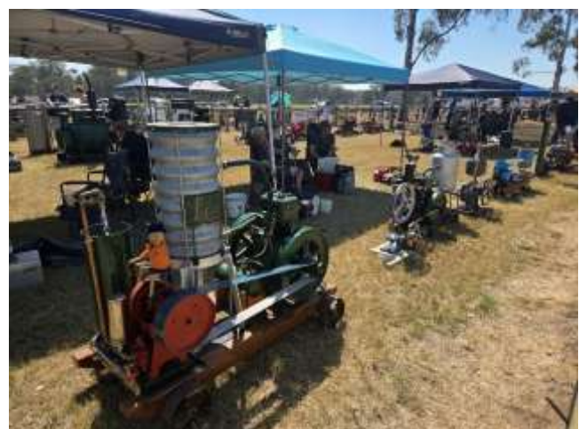
Ed's Lister A running a Nevertire/Sunshine water pump.
