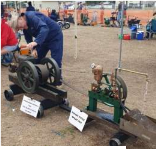
Kev's Root & Vandervoort engine used in the Childers District operating a Moffat Virtue Spraying Unit.
