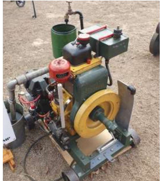
1961 Southern Cross EFD , 3.5hp with a Finsbury ½' Centrifugal Pump
