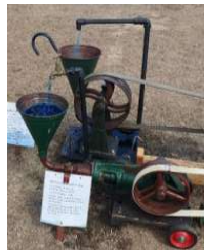
Ridd Milking Machine Vacuum Pump originally used in a Monto District Cream Dairy. This pump became obsolete when the dairy industry converted from cream production to bulk whole milk supply in about 1974.
