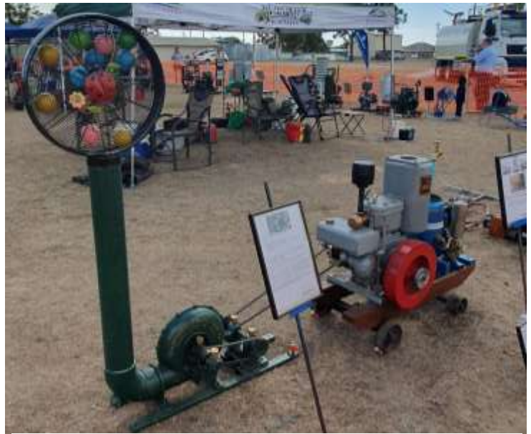
Jan's 1929 Type H "Ideal" engine with a Nevertire Piston Pump. The Champion No 1 Blower was made by Blower & Forge Co, Lancaster, USA in 1920's.
