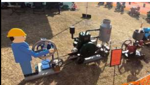
This Lister A series, 3hp, petrol, tank cooled engine was built circa 1937. This series of engines were built between 1923 and 1963. It is running a Nevertire / Sunshine water pump and was used mainly in the dairy industry.
