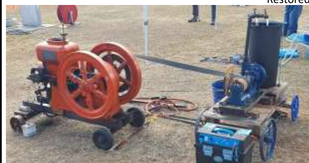
Made in US in 1916 and badged "Emu", it runs on a mixture of kerosene and petrol and was used to pump water from a well to a high level tank. Here it is working a Super Rapid 1 centrifugal pump. Restored by John.
