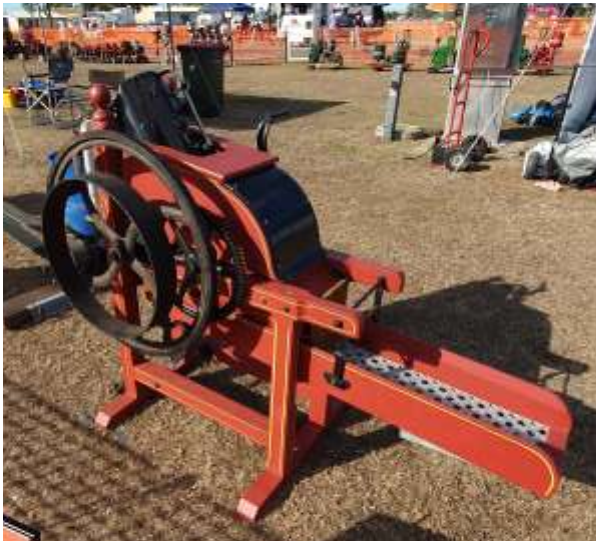
Bucsh's No 7 1/2 Two Hole Corn Sheller. It can be hand operated or belt driven. Original metal work circa 1899. The metal work and a single piece of timber was found in the back of a shed. The fully restored timber work was completed by owner, Ed.
