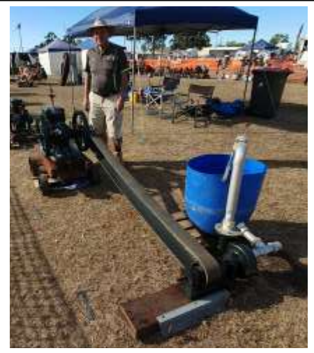
1923, 1 1/2hp IHC Model "M" engine . It has a low voltage internal ignitor. It's the last model before changing to spark plugs. Displayed by Laurie.
