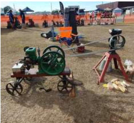
Keith's 1919 "Chore Boy", 1 3/4hp gasoline engine. 11 volt low tension ignition (no spark plugs)
