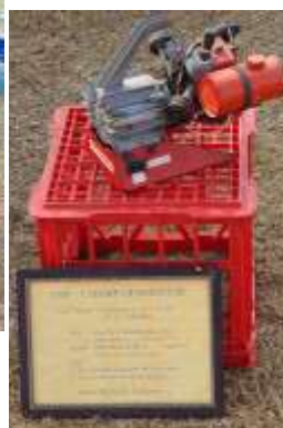
A Perry engine built in the early 1920's by Perry Engineering, Adelaide. 4hp petrol/kero likely used for cutting chaff for horses. Restored jointly by Vic and Todd Fauser.
