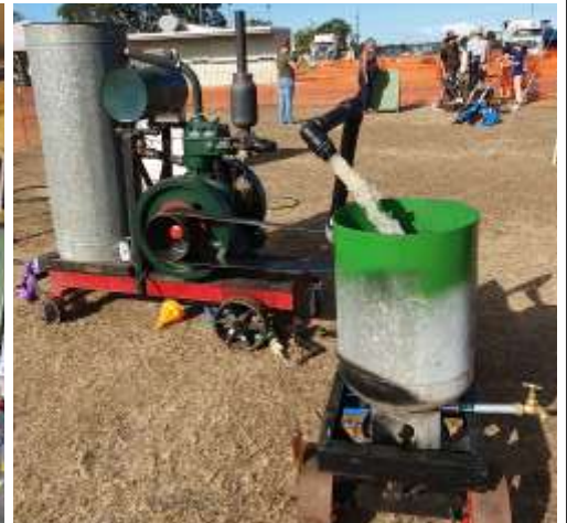
A 1927, 5hp Wolseley engine owned by Phil. This engine drove a line shaft in a shearing shed in Cooma.
