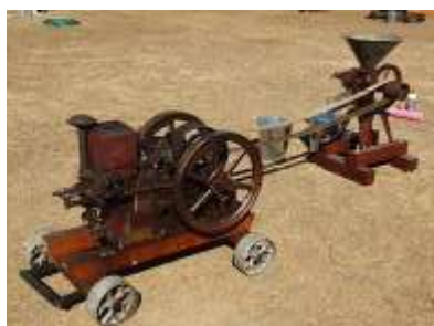
2hp United engine running a Cliff & Bunting grist mill
