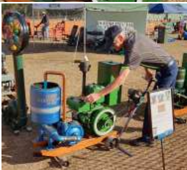
A Ronaldson & Tippet 3hp, Type N engine with a n IBC Centrifugal Pump
