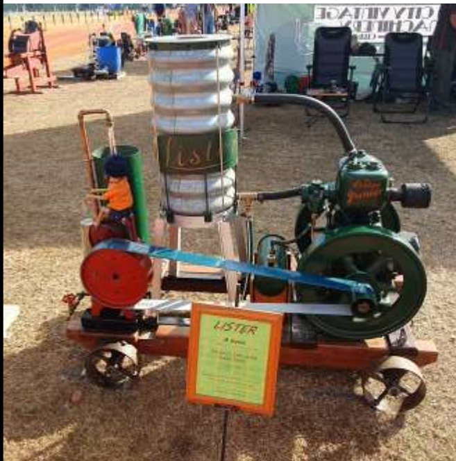
This Lister A series, 3hp, petrol, tank cooled engine was built circa 1937. This series of engines were built between 1923 and 1963. It is running a Nevertire / Sunshine water pump and was used mainly in the dairy industry.
