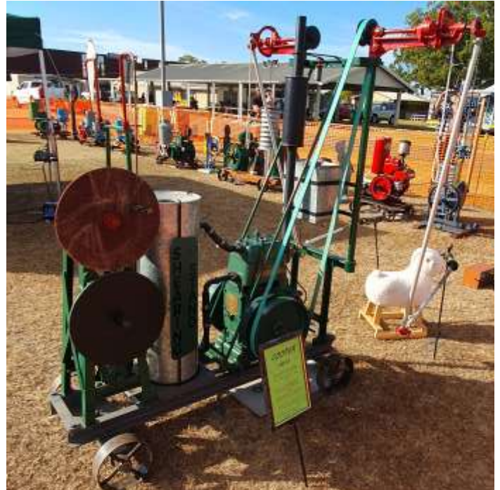
This Cooper XD, 4hp petrol, tank cooled engine was built circa 1959. Running twin grinding stations for the sharpening of shearing combs and used as a fixed or mobile shearing plant in the late 40's to early 60's, it was mainly used with smaller flocks in NSW and Vic. Fully restored and owned by Ed.
