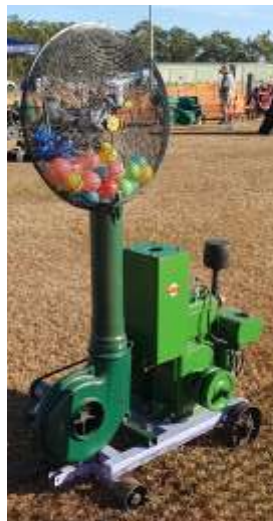
A Ronaldson & Tippet 3hp, Type N engine with a n IBC Centrifugal Pump
