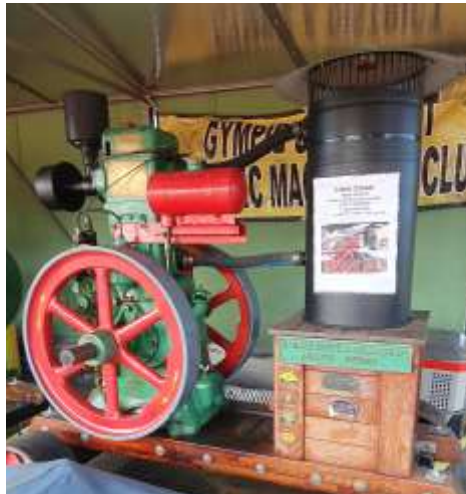
Mick's 1920 Lister Diesel, Model CS 6510. It's a water cooled single cylinder engine.
