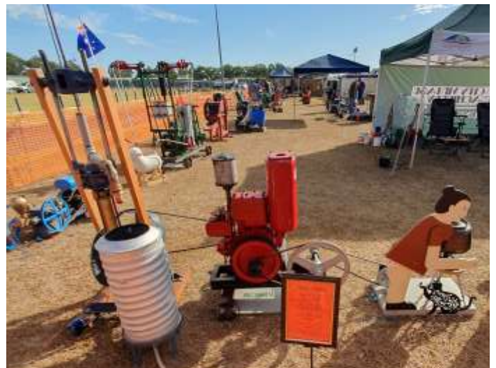
The Ideal 3hp type H engine was built circa 1948. It is a petrol/kero engine that is hopper cooled. It is badged International Harvester and was manufactured by Ronaldson & Tippet. It is running a Southern Cross Jack Pump.
