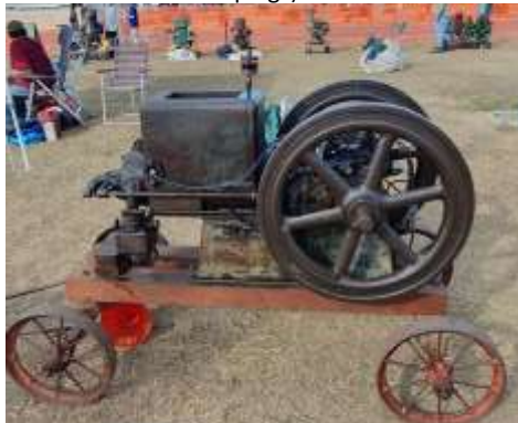
A Perry engine built in the early 1920's by Perry Engineering, Adelaide. 4hp petrol/kero likely used for cutting chaff for horses. Restored jointly by Vic and Todd Fauser.
