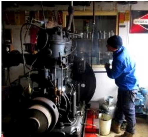
Here Simon inspects the engine before starting. There were two gas burners running flat out to heat the cylinder to get it to operating temperature.
