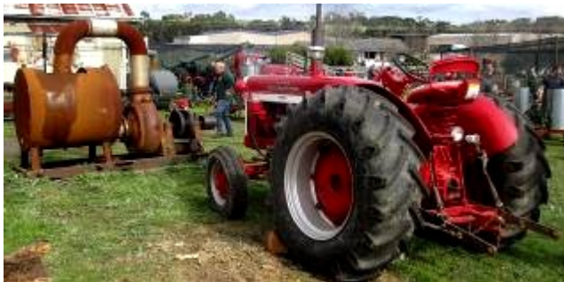
Tractor driving a huge centrifugal pump.
